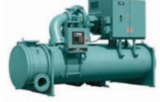
YK HP Water to water heat pump Centrifugal compr. / R134a Hot water up to 50°C (Std) Hot water up to 70°C (HP) Heating cap.: 1000 to 9000 kW
