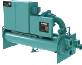
YMC² Water to water heat pump Variable speed centrif. compr. / R134a Magnetic bearings Hot water up to 65°C Heating cap.: 1600 to 3000 kW
