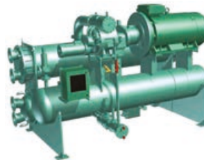
SHP Water to water heat pump Screw VSD compr. / R134a Hot water up to 80°C Heating cap.: 700 to 3000 kW
