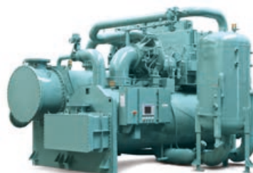
CYK HP Water to water heat pump Dual-Centrifugal compressors, Series-Arrangement / R134a Hot water up to 70°C Heating capacity from 2500 to 7000 kW
