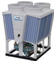
YHME Air to water HP Twin screw / R134a Hot water up to 55°C Heating capacity: 145 to 186 kW
