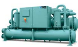
YVWA Water to water heat pump Screw compressor / R134a Hot water up to 65°C Heating cap.: 650 to 1250 kW
